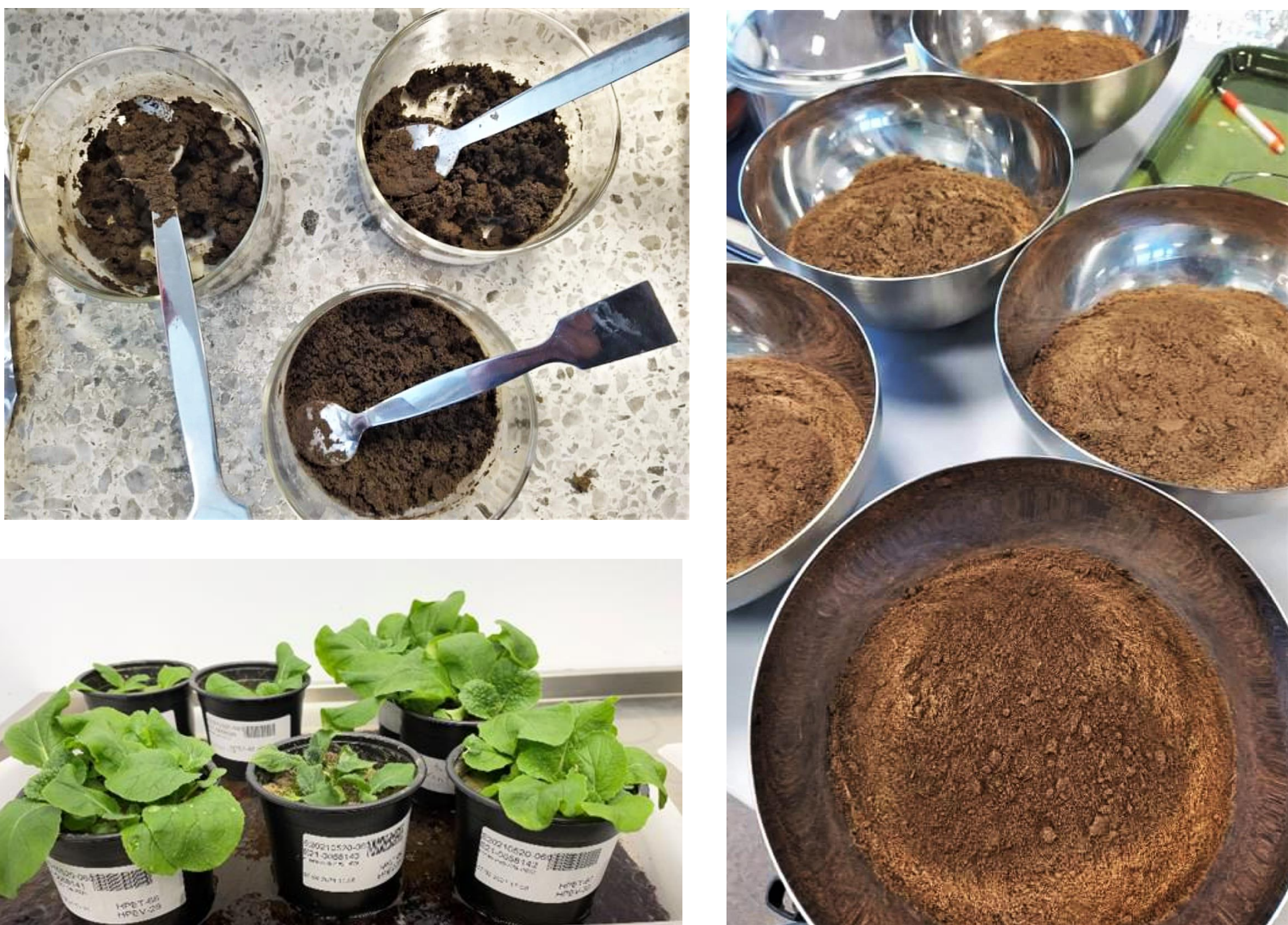
Figure 1. Soil and microplastic (< 3 mm) samples before mixture preparation. Plants grown in soil with added microplastic and determination of plant shoot fresh weight after 13 d growth. Photos: Liisa Maunuksela, Finnish Food Authority
